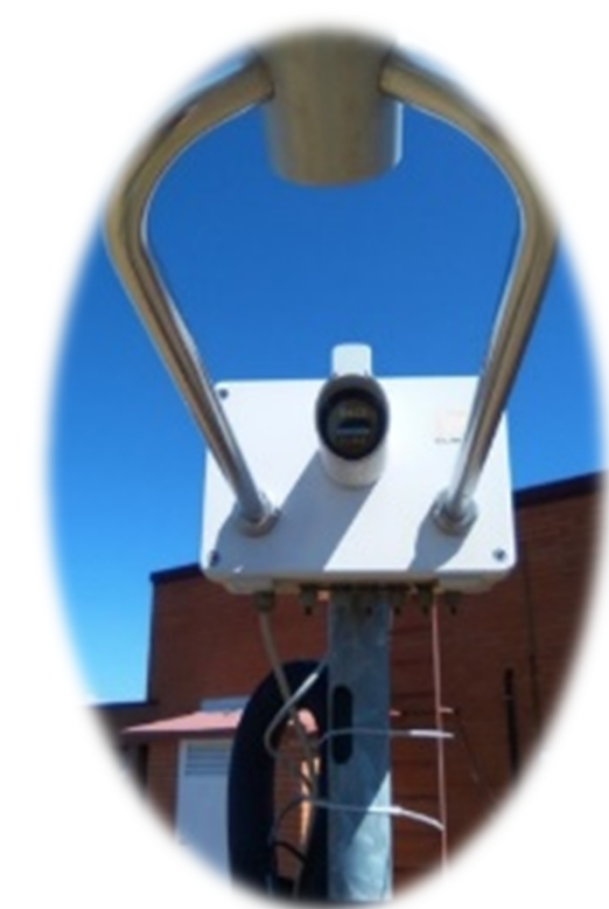
Fig. 2. Laser Precipitation Monitor (LMP) of Thies Clima used during the sampling campaign in León between January 2016 and December 2017.
