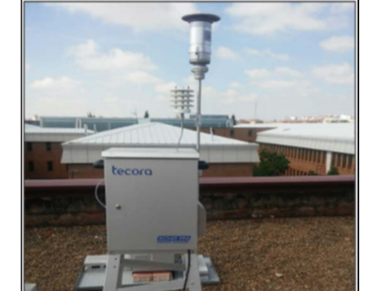
Low volume sampler (TECORA, ECHOPM): Collection of PM 10 (47 mm diameter teflon filters)
