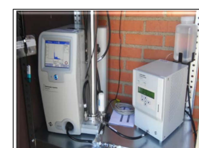
High resolution nanoparticle sizer (SMPS): Continuous monitoring of particle size distributions (0.018-1 µm)
