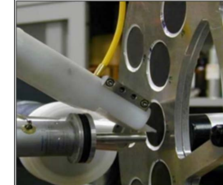
PIXE (Particle-Induced X-ray Emission): For the analysis of major and trace elements
