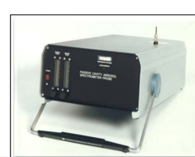
Optical particle counter (PCASP-X): Continuous monitoring of particle size distribution (0.1-10 µm)
