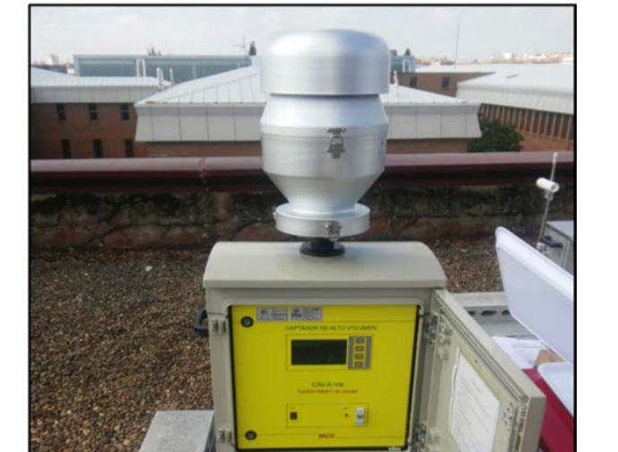
High volume sampler (CAV-A/Mb): Collection of PM 10 (150 mm diameter)
