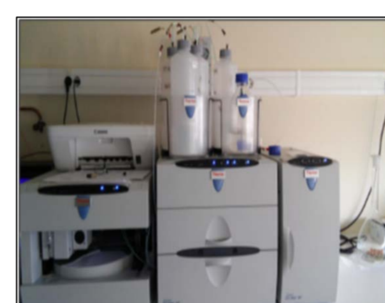
Thermo Scientific Dionex™ ICS-5000 Ion Chromatography: Analysis of water soluble ions
