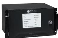
An aethalometer AE33 for measuring BC concentration, connected to TCA (using a slope EC:BC of 1).
